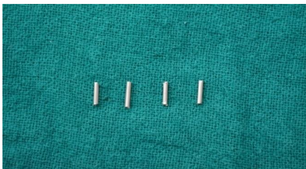
Fig 2: Steel tubes cut to the required length
