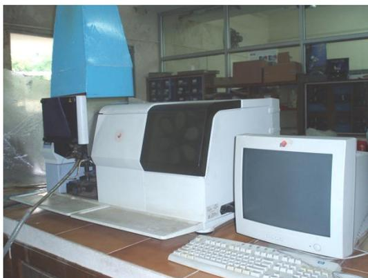
**Fig. 3: Atomic absorption spectrophotometry Unit**
