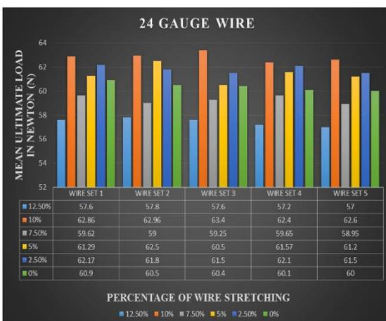
**Graph 1: Shows the graphical representation of 24 gauge wire mean ultimate load in Newton (N) with different percentage of stretching**
