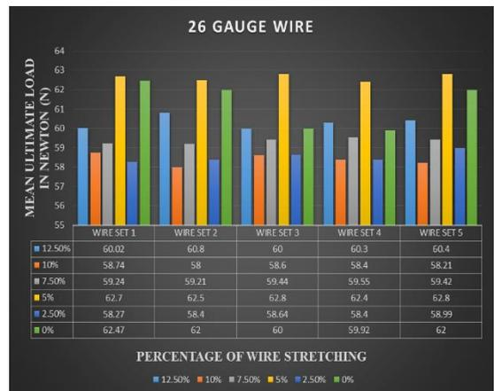
**Graph 2: Shows the graphical representation of 26 gauge wire mean ultimate load in Newton (N) with different percentage of stretching**
