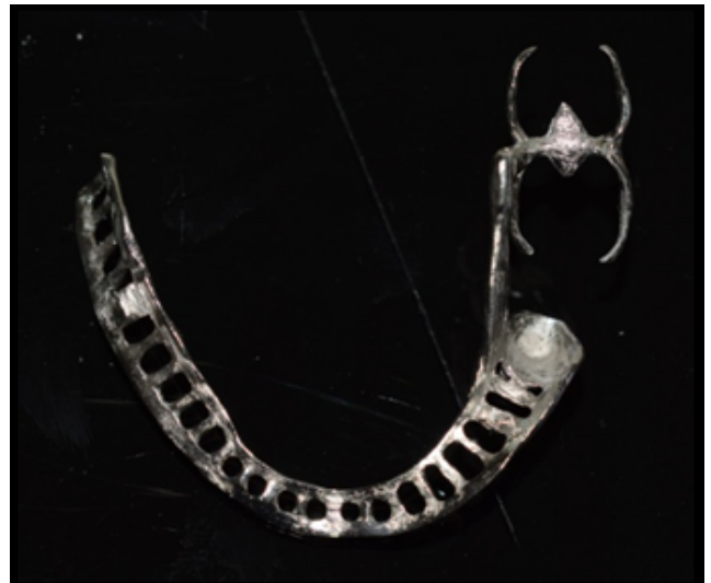
Fig. 7: Cast partial denture framework with hollow premolar
